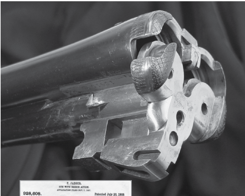
How the block slips in place. Note the groove on the lower left. The block pivoted around pins that protruded from both sides and allowed removal of the block when the barrel was taken off.
