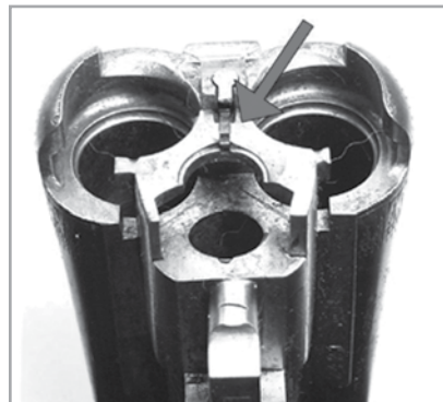
Here you can see the grooves in the underside of the integral barrel extension. The arrow points to a unique little feature, a lifter that pushes out the rifle cartridge a little farther for easy removal by hand.
